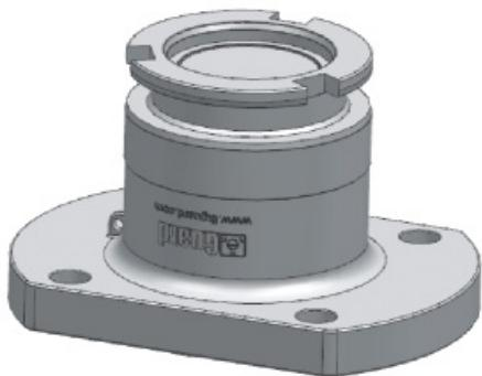
2 1/2 " dry joint - inlet flange of  $4 \times \phi 17$  are all distributed on the PCD160mm flange surface, the outlet is  $\phi 104.7$ mm joint, the main seal is made of Vition material sealing ring, in addition, DN80,DN50 product specifications can be selected.
