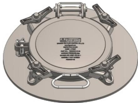
DN250 Inspection 4 points, 8mm thickness, 8mm thick flanged low profile is welded and formed. The maximum opening angle of the cover is 135° or 120°. Can be used as injection port. Seal sold separately.
